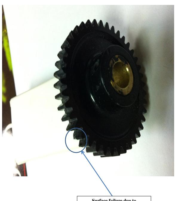
Surface failure due to misalignment of load
