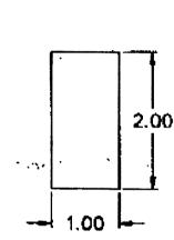
Construct a solid box 2 units long by 1 unit wide and 1 unit in height using the Box command. Begin this box at absolute coordinate 5.5,1.5. This slab will represent the rectangular hole made into the slab that will be subtracted at a later time.
