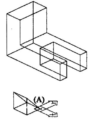
The wedge needs to be rotated 90 degrees about the X axis before being placed into position and subtracted from the main solid. Use 3drotate command to accomplish this. once in the command, a new icon appears: it is Motion
