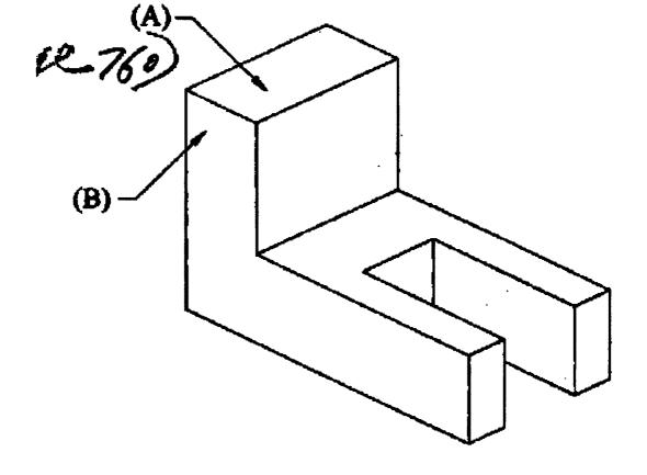
Using the Hide command perform a hidden line removal on all surfaces of the object. Th results are illustrated at right.
