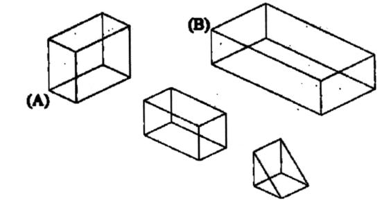
Use the Union command to join the base and the vertical column into one entity
