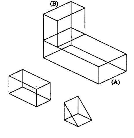
Use the Move command to position the rectangle from its midpoint at "A" to the midpoint of the base at "B". In a moment, the small rectangle will be subtracted forming the rectangular hole in the base.
