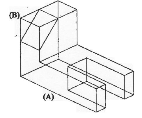
An alternate method of creating the inclined surface is to use the Chamfer command to chamfer the vertical column.
