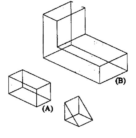
Use the Subtract command to subtract the small rectangle from the base of the solid.
