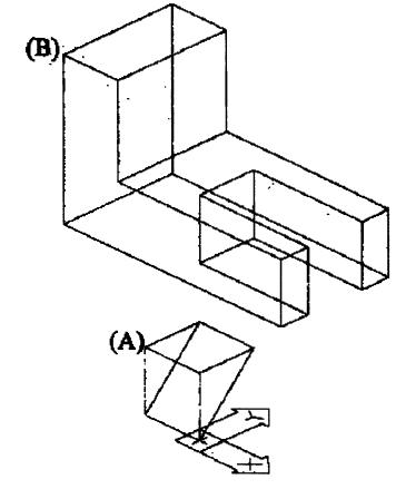
Use the Subtract command to subtract the wedge from the main solid.
