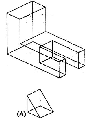
Move the coordinate system icon to a new origin located on the wedge
