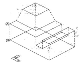
Repeat the above procedure to connect the remaining edges of the wire-frame model. When completed, set the Osnap command to None.
