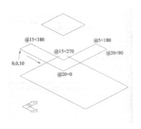
Construct the next surface of the wedge using the following prompts of the Line command:
