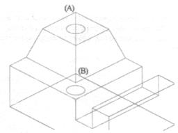
Use the Circle command again to place the circles of diameters 2.00 in the slot as illustrated at right. Use the absolute coordinates of 22.5,5,5 and 22.5,15,5 to identify the centers of the circles.
