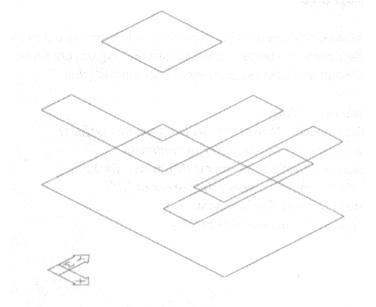
Use the Line commnad to connect the all levels to complete the outline of the Wedge. Be sure to use Osnap-Endpoint option at all times.
