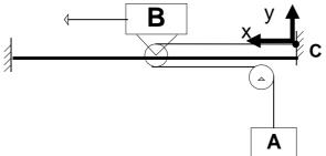
moves to the left at  $v_B = 3$  m/s, and accelerates also to the left at  $a_B = 0.5$  m/s<sup>2</sup>. Using the x-y frame with origin at C, determine: (a) the velocity of A
