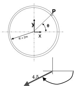
**3.** (20 points) Pin P moves at constant speed of 3 m/s in a counterclockwise sense around the circular slot with radius r = 2 m. Determine (a) the angular velocity of P. (b) the total acceleration **vector** (Use polar coordinates:  $e_r$  and  $e_{\theta}$  directions) of pin P when  $\theta = 30$  degrees. (c) the magnitude and angle of the resultant acceleration vector in **Cartesian** x-y coordinates.
