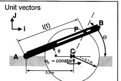
Determine the angular velocity of arm AB as  $\Theta = 90$  degrees.
