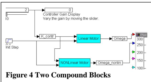
**Getting Real: Nonlinearities** - Duplicate the compound block 'Linear Motor' and rename it 'Nonlinear Motor'. Connect 'Nonlinear Motor' to inputs K\_contr and unit step, and to a new output Omega\_nonlin, connect Omega\_nonlin to the plot. See Fig. 4. Edit the nonlinear block and insert the following nonlinearities from the Blocks → Nonlinear menu:
