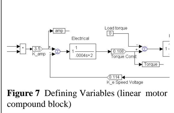
**(c) Effect of Load Torques** – All simulations above were conducted with zero loads. Enter the same small non-zero load in each compound block and observe the motor performance. Do NOT let the motor run backwards (negative speeds). Plot a nice example of driving a load.
