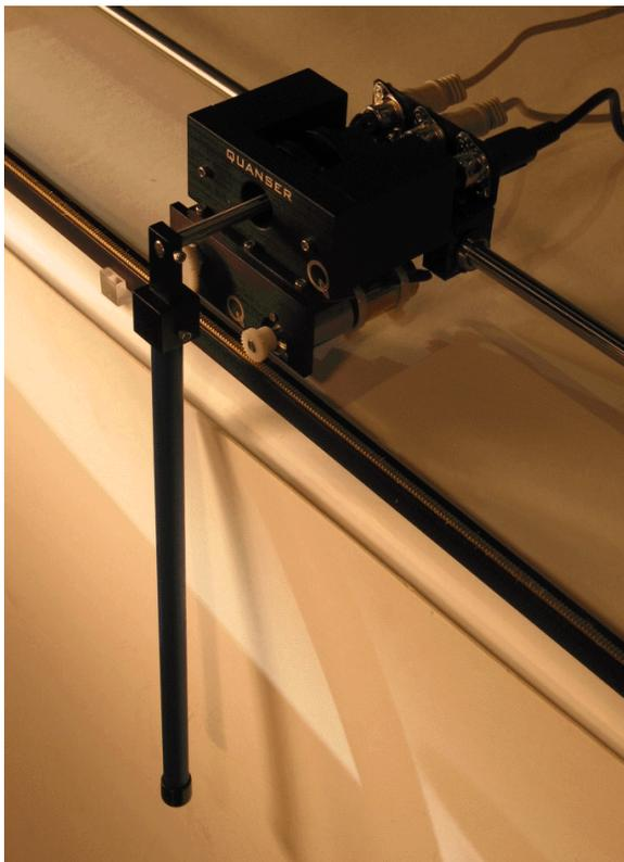
Figure 1 Medium Pendulum Suspended in Front of the IP02
