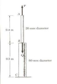
2.17 Both portions of the rod ABC are made of an aluminum for which E = 70 GPa. Knowing that the magnitude of P is 4 kN, determine (a) the value of Q so that the deflection at A is zero, (b) the corresponding deflection of B.
