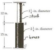
2.52 A rod consisting of two cylindrical portions AB and BC is restrained at both ends. Portion AB is made of steel ( $E_s = 29 \times 10^6$  psi,  $\alpha_s = 6.5 \times 10^{-6}$ )°F) and portion BC is made of brass ( $E_b = 17 \times 10^6$  psi,  $\alpha_b = 10.4 \times 10^{-6}$ ). Knowing that the rod is initially unstressed, determine (a) the normal stresses induced in portions AB and BC by a temperature rise of 65°F, (b) the corresponding deflection of point B.
