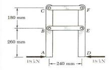
**2.25** Members ABC and DEF are joined with steel links (E = 200 GPa). Each of the links is made of a pair of  $25 \times 35$ -mm plates. Determine the change in length of (a) member BE, (b) member CF.
