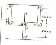
**2.41** Three steel rods (E = 200 GPa) support a 36-kN load **P**. Each of the rods AB and CD has a 200-mm<sup>2</sup> cross-sectional area and rod EF has a 625- mm<sup>2</sup> crosssectional area. Determine the (a) the change in length of rod EF, (b) the stress in
