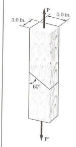
**1.31** The 1.4 kip load **P** is supported by two wooden members of uniform cross section that are joined by the simple glued scarf splice shown. Determine the normal and shearing stresses in the glued splice.
