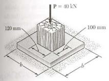
1.20 A 40-kN axial load is applied to a short wooden post that is supported by a concrete footing resting on undisturbed soil. Determine (a) the maximum bearing stress on the concrete footing, (b) the size of the footing for which the average bearing stress in the soil is 145 kPa.
