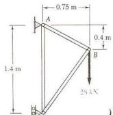
1.41 Members AB and BC of the truss shown are made of the same alloy. It is known that a 20-mm-square bar of the same alloy was tested to failure and that an ultimate load of 120 kN was recorded. If a factor of safety of 3.2 is to be achieved for both bars, determine the required cross-sectional area of (a) bar AB, (b) bar AC.
