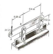
**1.9** Each of the four vertical links has an  $8 \times 36$ - mm uniform rectangular cross section and each of the four pins has a 16- mm diameter. Determine the maximum value of the average normal stress in the links connecting (a) points B and D, (b) points C and E.
