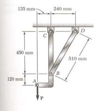
1.7 Knowing that the central portion of the link BD has a uniform cross-sectional area of 800 mm2, determine the magnitude of the load P for which the normal stress in that portion of BD is 50 MPa.
